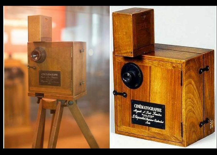
Much smaller and lighter than Edison's Kinetograph, le cinématographe Lumière weighed around 11 pounds and operated with the use of a hand-powered crank.
