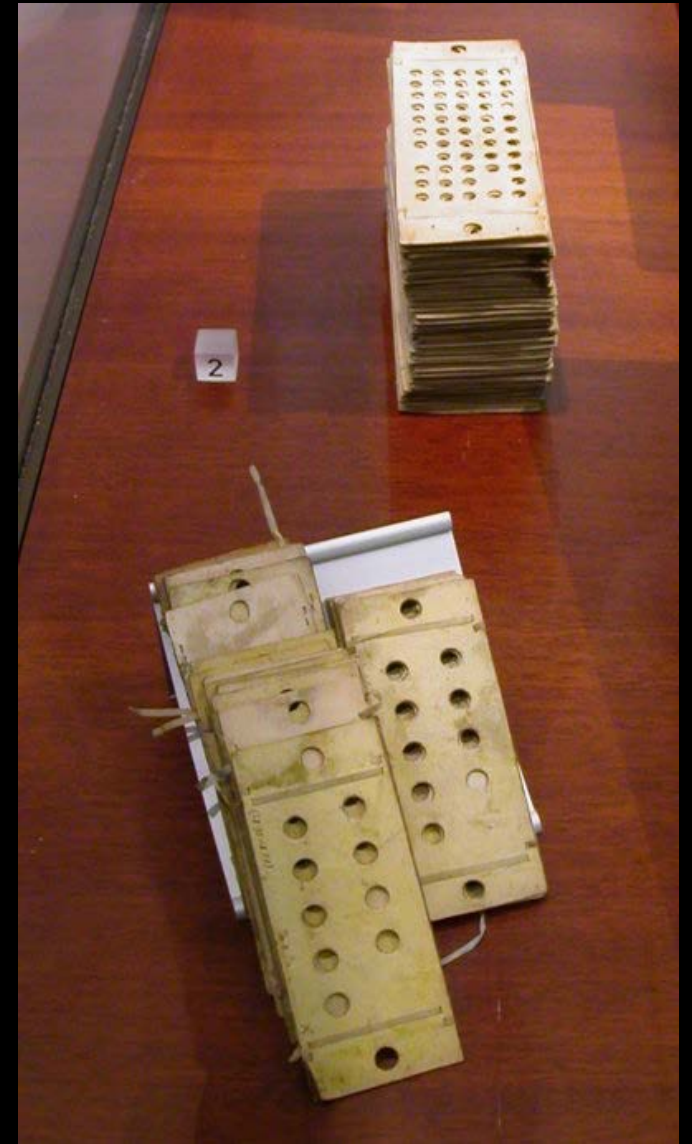
Two Types of Punch Cards Used to Program His Analytical Engine of 1837
